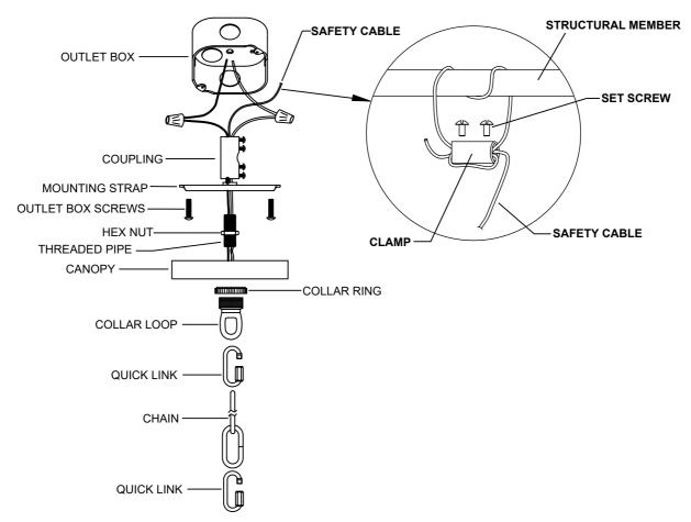
NOTE:NEC CODE (314.24) requires that ceiling outlet boxes in the United States support up to 50 lbs. This fixture exceeds 50 lbs. and must be installed using an outlet box approved for up to 100 lbs. or independently of the existing outlet box. Installation hardware and instructions are provided for both.
