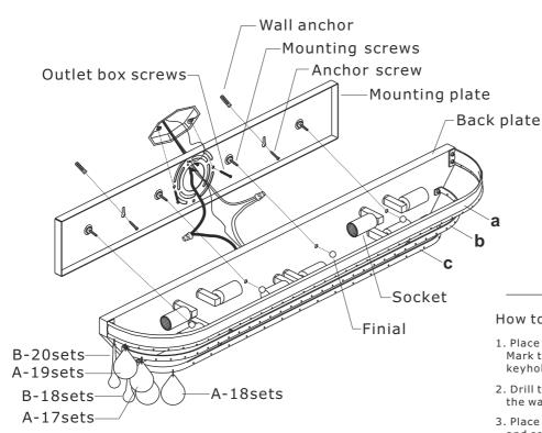
Hang crystals to rings "a" and "b" alternating between crystals A and B. Hang crystal A to ring "c".
